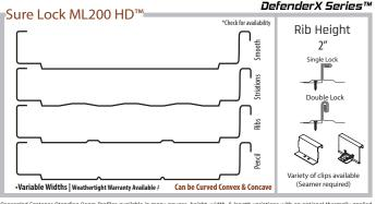
Concealed Fastener Standing Seam Profiles available in many gauges, height, width, & length variations with an optional thermally-applied butyl Sure Seam Sediant\*\* available for low slope applications. Weathertight Warranties Available, Please inquire for more information.
