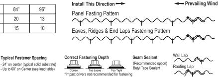
\*The above diagrams are the typical fastener pattern based on the live load table. However pattern & spacing may not be appropriate for all applications. Consult local building codes and/or professional engineer for alternative use
