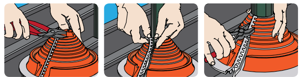
1. Using tin snips, cut the cone to fit pipe.
