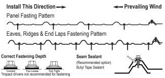
\*The above diagrams are the typical fastener pattern based on the live load table. However pattern & spacing may not be appropriate for all applications. Consult local building codes and/or professional engineer for alternative use.
